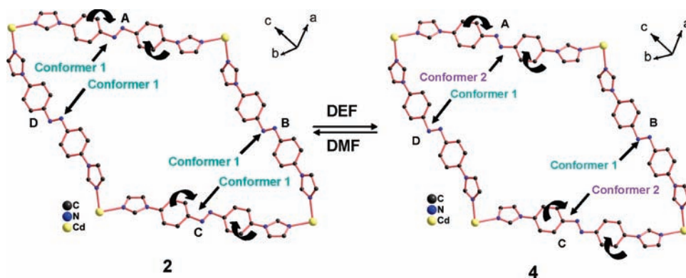
Figure 8. Schematic representation of reversible SC–SC pedal motion in compound 2 after DEF/DMF exchange (guest molecules are removed for clarity).
